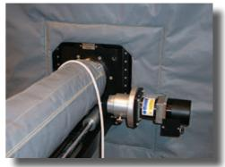
Heating jackets are often used in combination with heating tents to cover the protruding components, such as a Manipulator bellow.
